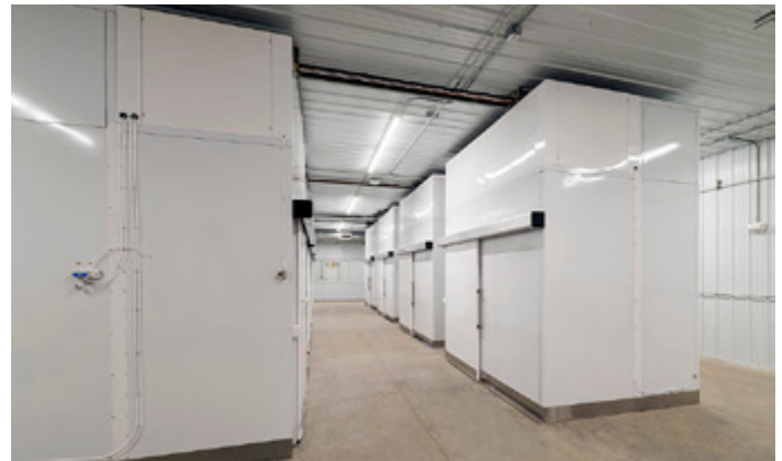
Percival environmental control chambers awaiting placement of the robotic arm. The arm will move between each chamber and access the research materials through the sliding doors on each chamber.
